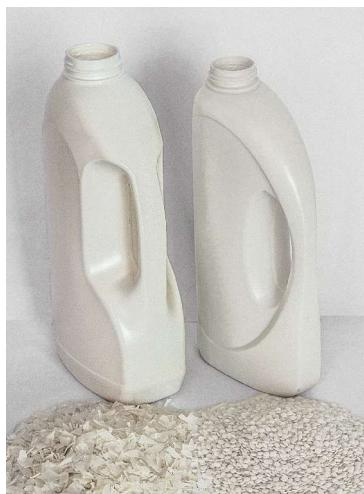
Feedstock for the test came from post-consumer detergent bottles that had retained a persistent odor of dishwashing or laundry detergent even after shredding and washing. The goal of the project was to produce odor-free regrunulate with properties comparable to virgin material.
